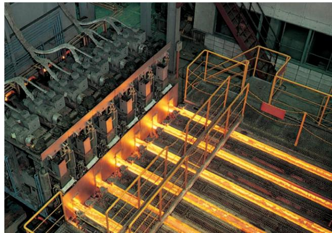
連続 casting Continuous casting
